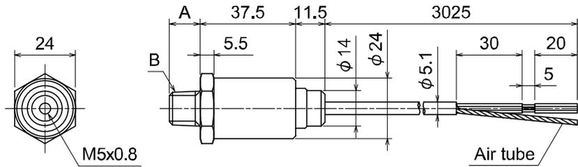
Be sure to release the air in the air tube of the cable to the atmosphere.
