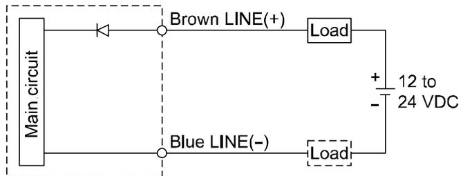
\*: Install the load either on the LINE(+) or LINE(-) side.
