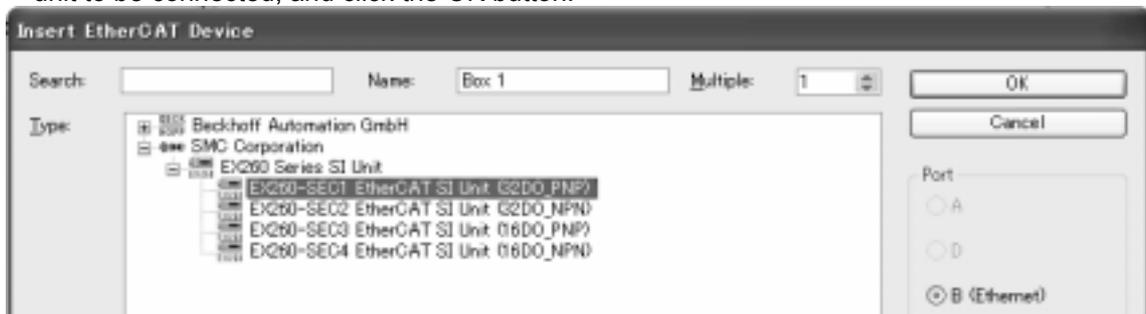
\*: If EX260 Series SI unit is not found in the list, confirm whether the XML file of this unit is in the [TwinCAT\IO\EtherCAT] folder, and start up [TwinCAT( System Manager)] again
