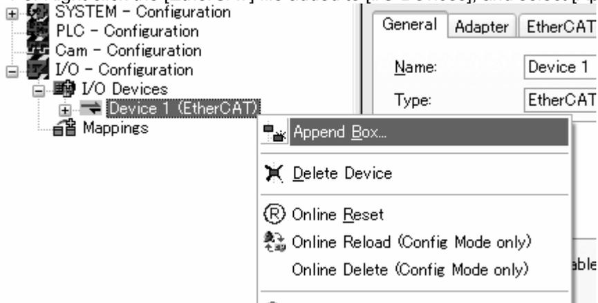
2-1-4. After clicking the [SMC Corporation] and [EX260 Series SI Unit] files in sequence, select the unit to be connected, and click the OK button.
