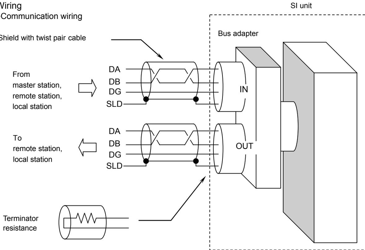
Connect the terminal resistance to the end of connection on the network.
